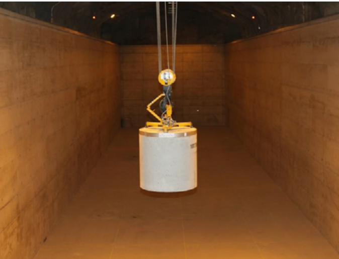
Figure 4-15. The transfer of the first solidified waste container into the concrete basin in the solidified waste hall in December 2019.
